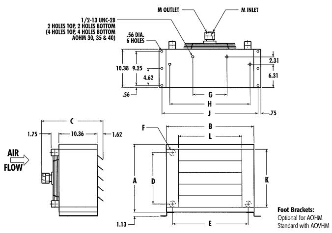
See dimensional chart for external NPT or optional internal SAE connection size.
