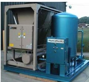
**Packaged pump and control skid.** Pumps, electrical enclosure, vent and surge tank, piping, valves, gauges, wiring and thermostatic spray pump control are all completely factory assembled on a full-deck fabricated steel base.
